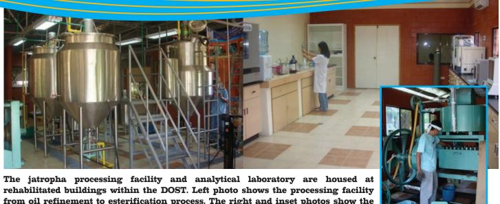
from oil refinement to esterification process. The right and inset photos show the laboratory set-up for analysis of Jatropha properties, and Jatropha seed expeller for jatropha methyl ester production, respectively.
