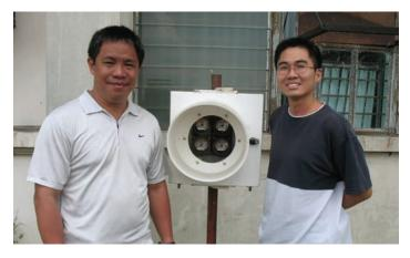
The project "An Improved Air Pollution Sensor Utilizing Differential Optical Absorption Spectroscopy Technology" developed an instrument that measures ambient concentrations of sulfur dioxide, ozone and nitrogen dioxide. Shown in the photo are project leader Dr. James B. Simpas with research assistant Sherdon Niño Y. Uy beside the retroreflector.
