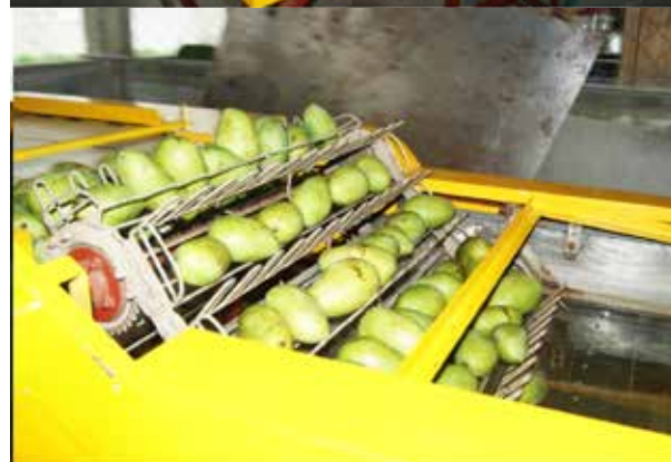
Automated hot water treatment for mangoes was developed by a group of engineers from Mariano Marcos State University.
