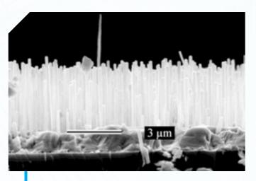
The ongoing project "Nanostructured Solar Energy Devices" aims to develop new innovations in solar cell energy research based on nanotechnology. Photo shows a scanning electron microscope image of Gallium Arsenide (GaAs) nanowires on silicon substrates produced via molecular beam epitaxy. GaAs nanowires enhance solar cell performance.
