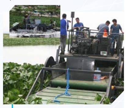
A group of technicians from the Metro Manila Development Authority tested the harvester at a swamp near the Taguig Pumping Station. The harvester was developed to collect free-floating water hyacinth by cutting them onsite and conveying them to the platform hold.
