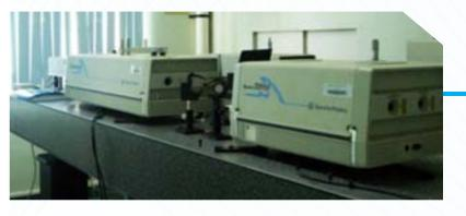
In 2011, PCIEERD supported the laboratory upgrading of the National Institute of Physics (NIP) of the University of the Philippines Diliman. Through the funding assistance, NIP will upgrade its femtosecond laser facility to be able to perform terahertz time-domain spectroscopy. Shown in the photo are the current femtosecond laser and frequency doubler at NIP.
