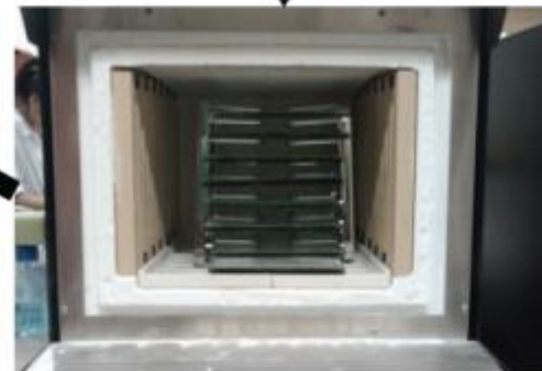
Blasting of 8 glass plates in a furnace at 300°C
