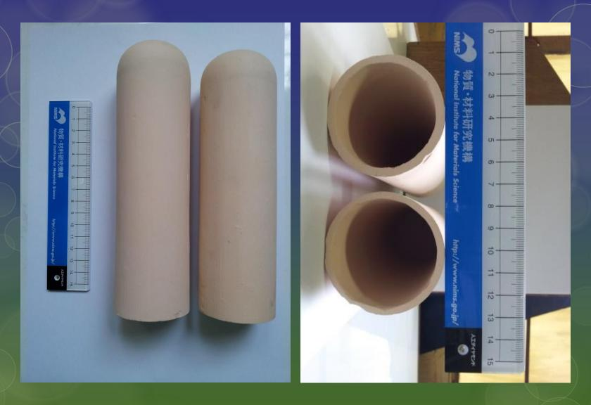
$1^{\rm st}$  generation ceramic filter units (max.  $300 \, \rm mL/min$ ); ~25 cm tall; ~5 cm diameter & ~5 mm thick.
