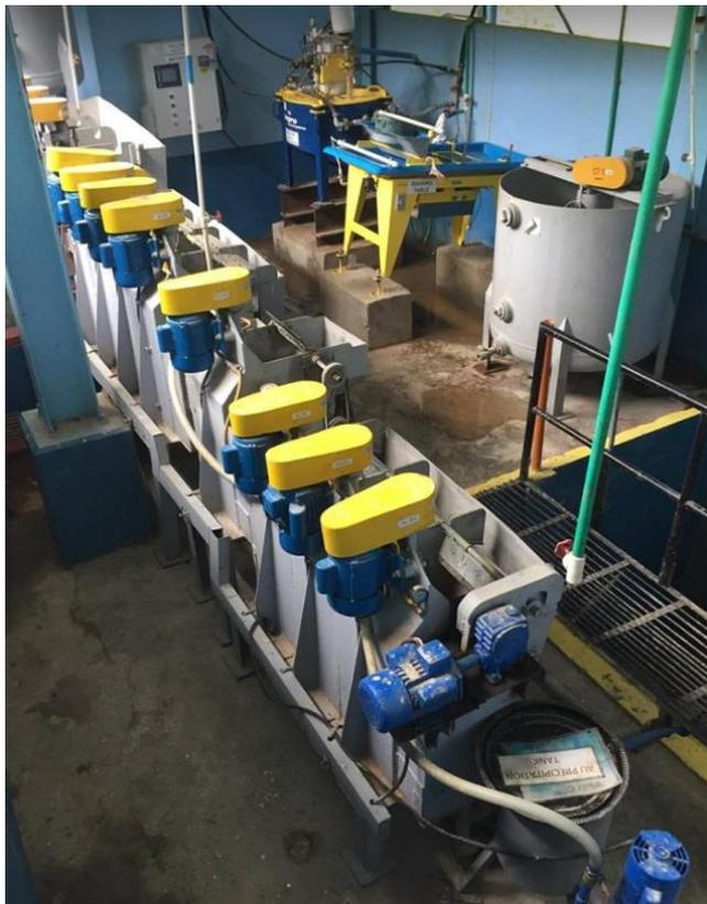
Fig. 2. Flotation cells and gravity concentrators
